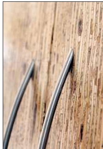
CanWest News Service Kirei board is made from the stalks of sorghum plants.
